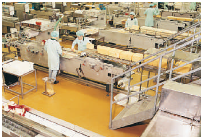
Specifically developed for the food, beverage and pharmaceutical industries, UCRETE® DP meets the requirements of the U.S., European and Australian standards for slip resistant pedestrian surfaces.
